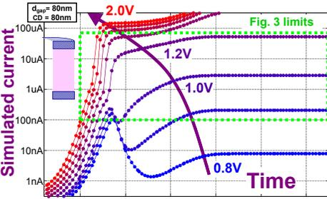
**Fig. 12** Transient simulations of MIEC AD response show that the ion migration needed to turn on an MIEC AD occurs slowly at low bias and current, yet rapidly at high bias and current, although not with the same wide dynamic range observed in experiments (Fig. 3). Transient data at higher temperature is likely to be faster, accommodated by adjusting the rate constants in Figs. 4 & 7 with the appropriate energy barriers.
