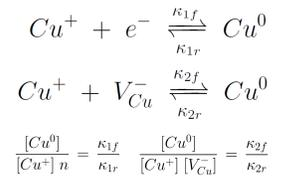
**Fig. 4** Sentaurus TCAD [6] is used to model drift, diffusion, and two rate-equation interactions between mobile copper ions ( $Cu^+$ ), atoms ( $Cu^0$ ), mobile vacancies ( $V_{Cu}^-$ ), and electrons.
