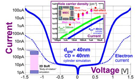
**Fig. 8** Simulated IV curve for a cylindrical MIEC AD. As bias increases, electron-dominated current gives way to holes, matching Hall-effect measurements (inset).
