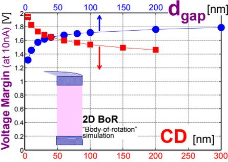
**Fig. 10** Variation in simulated voltage margin as thickness ( $d_{gap}$ ) and diameter (CD) vary around the CD = 40nm,  $d_{gap}$  = 40nm cylinder shown in Fig. 8.
