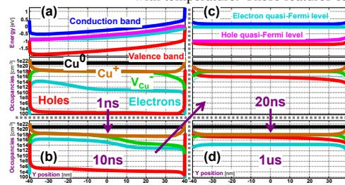
**Fig. 13** After a voltage ramp to 1.0V (a, 1ns), hole occupancy remains suppressed by the large  $Cu^+$  population diffusing slowly away from the positive (left) interface (b, 10ns). After 20ns (c), this ion population has departed, flattening the bands and allowing some hole injection. By 1us (d), the slow interaction between  $Cu^+$  and electrons has suppressed electron current, allowing hole current to dominate.
