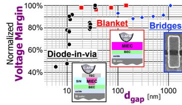
**Fig. 2** Measured turn-on voltages depend strongly on device CD [2] (not shown), but are insensitive to the gap between electrodes ( $d_{gap}$ ) down to very small thicknesses.
