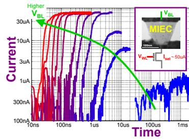
**Fig. 3** Larger applied voltages with higher saturation currents lead to faster turn-on of MIEC access devices.
