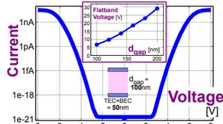
**Fig. 6** While a simulated MSM structure without ions has an MIEC-like IV, currents are too low and ON-transition voltages are large and depend strongly on  $d_{gap}$ .
