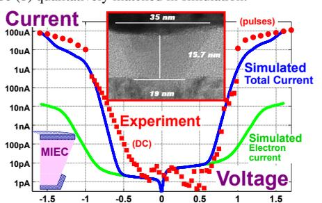
**Fig. 14** By carefully tuning the simulation mesh against TEM images for dimensions and the slight recess into the bottom electrode, precise matching of IV characteristics can be obtained, including ultra-low leakage currents, voltage turn-ON values, and >7 orders of magnitude in ON-OFF ratio.
