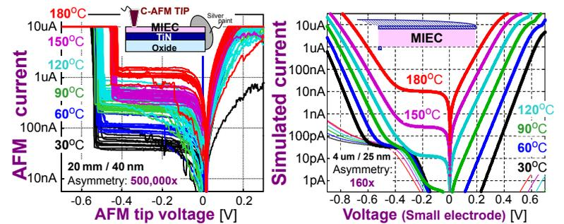
**Fig. 11** (a) Conductive-AFM measurements of blanket films show highly asymmetric IV characteristics because of the large asymmetry in electrode areas, and noise floor increases with temperature. These features can be (b) qualitatively matched in simulation.
