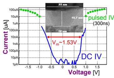
**Fig. 1** Access Devices (ADs) based on Cu-containing Mixed-Ionic-Electronic-Conduction (MIEC) materials exhibit bipolar diode-like characteristics with ultra-low leakage and large ON/OFF ratios [1-5].
