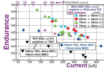
Fig. 9 ADs show better endurance as the thickness, and thus the volume from which  $\text{Cu}^+$  is accumulated during cycling (see Fig. 11), becomes smaller.
