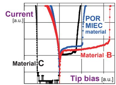
Fig. 14 Conductive-AFM measurements (small-area tip on various MIEC materials on unpatterned BEC) provide early guidance on the  $V_m$  (but not on leakage current) to be expected from wide-area TEC ADs.
