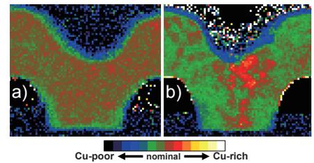
Fig. 11 Local stoichiometry from TEM/EELS of wide-area TEC, 80nm BEC ADs a) as-fabricated, and b) after 425,000 cycles at  $325 \mu\text{A}$ . Regions near the TEC (biased negative for cycling) have become markedly Cu-rich.
