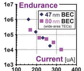
Fig. 8 MIEC-based AD endurance depends on current, but is independent of BEC CD, despite the nearly 3-fold change in current density.
