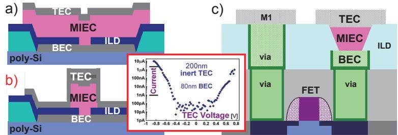
Fig. 2 MIEC-based ADs with non-ionizable electrodes are fabricated on 4'' wafers with a) wide-area TECs ( $\gg$  BEC), b) TECs patterned to enable bipolar operation (inset) with ion-milling, and c) on 8'' wafers with integrated FETs using Chemical-Mechanical Polishing (CMP).
