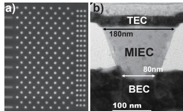
Fig. 4 a) Top-down view of metal- and MIEC-vias for a  $5 \times 10$  array (w/ dummy rows/columns), after CMP; (b) TEM cross-section of a Diode-In-Via (DIV) AD, with planarized MIEC material capped by the TEC.
