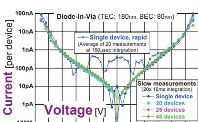
Fig. 6 Slow measurements, performed on single or multiple all-good devices, reveal that leakage currents in MIEC-based ADs near 0V are  $< 10$  pA.
