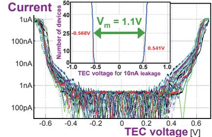
Fig. 5 Measured i-v characteristics for a  $5 \times 10$  array of DIV ADs, tested with integrated FETs, showing large voltage margin ( $V_m \sim 1.1$ V) and tight distributions.
