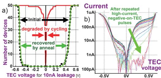
Fig. 12 Low-leakage i-v characteristics that have been degraded by endurance failure or high-current pulses can be recovered by either a) thermal annealing, or b) high-current pulses of the opposite polarity. This implies that local accumulations of Cu shown in Fig. 11 can be successfully redistributed.
