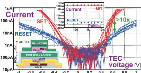
Fig. 3 Cycling of a 33nm pore-cell PCM, with SET, RESET, and read performed through an overlying AD (80nm BEC), which showed no degradation despite the  $> 10^4$  high-current pulses. The 200nm TEC allowed “good polarity” (positive-on-TEC) PCM operation [7].
