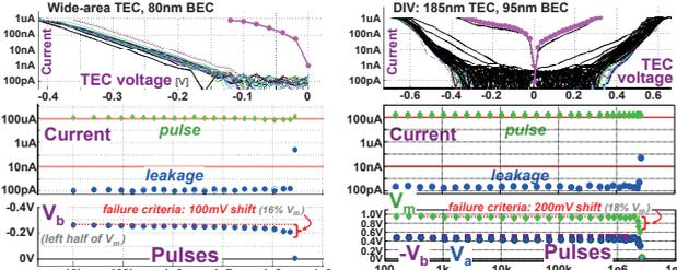
Fig. 7 Both a) wide-area TEC and b) DIV MIEC-based ADs can operate without degradation for many high-current pulses, but eventually a change from low- to high-leakage occurs. This change is abrupt in all but the thickest ADs.
