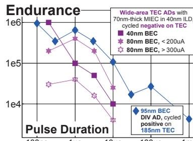
Fig. 10 For both wide-area TEC and DIV ADs, endurance improves as pulse duration is reduced.
