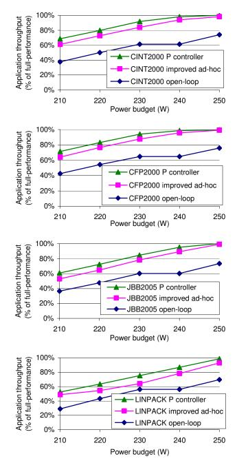
**Figure 9: Application performance.** The Y-axis shows throughput performance compared to the application running at full-performance (no power management).
