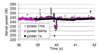
**Figure 6: Linpack without power management.** Graph shows 4 seconds of the Linpack benchmark after running for 38 seconds. Average power over 1 ms, 64 ms, and 1 s periods is plotted. The plot points mark the end of the measurement period. Linpack has almost constant power consumption with periodic dips in power (as seen around the 40 second mark).
