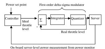
Figure 3: System diagram for power control
