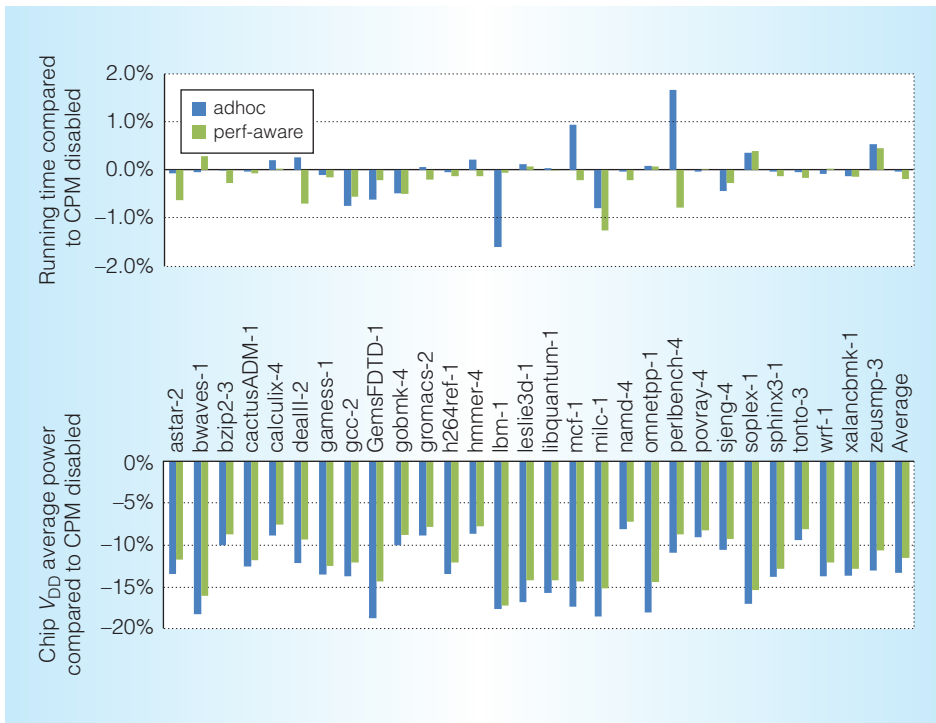
Figure 7. Comparison of undervolting algorithms to CPM disabled. The top graph shows the workload’s average running time (lower is better). The bottom graph shows the average Power7+ V_{DD} rail power (lower is better). The number after each benchmark name signifies the number of hardware threads on each core running the workload.
