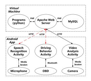
Fig. 7. The system design of SafeShareRide.
