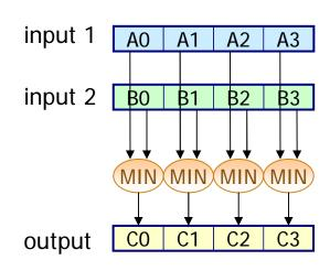
Limitation: SIMD load / store instructions can be effective only when they access contiguous 128 bits of data (e.g. four 32-bit values) aligned on 128-bit boundary
