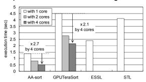
Figure 12. The execution time of parallel versions of AA-sort and GPUTeraSort on up to 4 cores of PowerPC 970MP.
