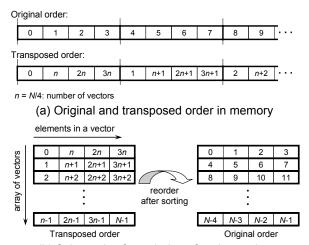
(b) Schematic of reordering after the sorting **Figure 3. Transposed order.**
