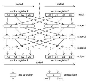
Figure 6. Data flow of vector merge operation.
