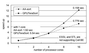
Figure 13. Scalability with increasing number of cores on Cell BE for 32 million integers.
