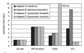
Figure 11. Performance comparison on one PowerPC 970MP core for various input datasets with 32 million integers.
