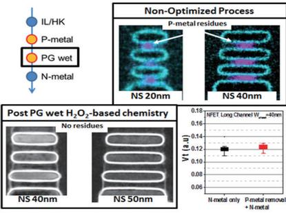
Fig. 13: P-metal can be fully removed in wide Nanosheet structures using  $H_2O_2$ -based chemistry with no impact on the structure and gate stack properties
