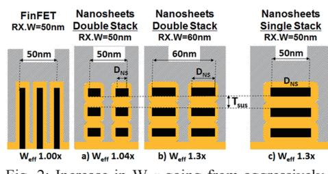
Fig. 2: Increase in  $W_{eff}$  going from aggressively scaled FinFET to double and single stack Nanosheets structures. Best improvement is obtained using a single wide Nanosheet stack at constant active width (RX.W).
