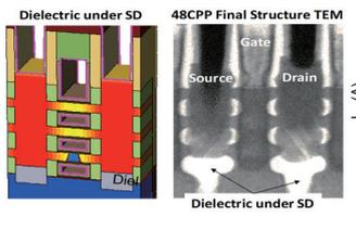
Fig. 15: Sub-sheet leakage suppression when a dielectric is inserted under the source/drain, comparable to fully isolated.
