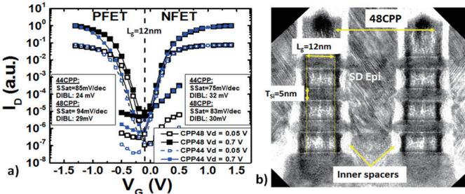
Fig. 11: Stacked Nanosheet 44/48nm CPP nFET/pFET devices  $I_D/V_G$  - Structures feature 3 sheets, inner spacer,  $L_g=12nm$ , and  $T_s=5nm$
