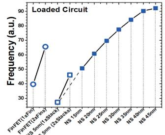
Fig. 6: Inverter driving a capacitive load. Performance of a single wide Nanosheet stack is superior. Note: improved granularity for power optimization.
