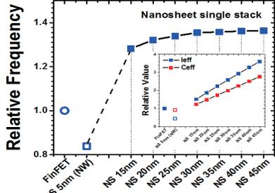
Fig. 5: Relative Frequency for several device options: FinFET, Nanosheet 5nm (Nanowire), and various widths single stack Nanosheets. Inset:  $C_{eff}$  and  $I_{eff}$  for same devices.
