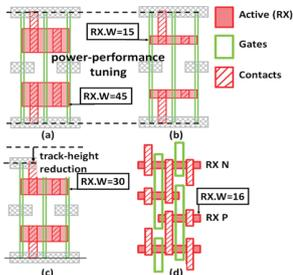
Fig. 4: For a given cell height, the Nanosheet (RX) width can be varied to optimize power-performance trade-offs in logic (a-c) and SRAM (d).
