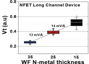
Fig. 14: nFET long channel  $V_t$  modulation with N-metal
