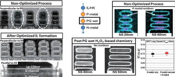
Fig. 12: Stiction between Nanosheets is suppressed with optimized IL formation
